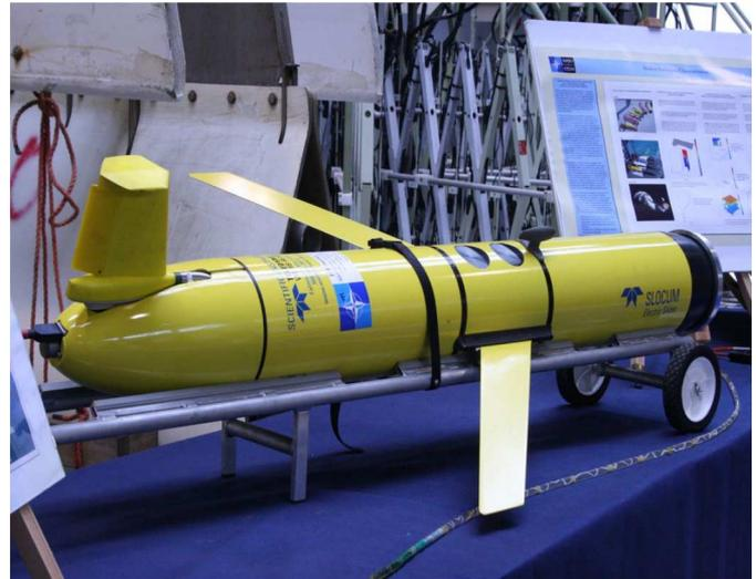
Fig. 1. Slocum glider recently acquired by NURC. The picture shows the Slocum glider with the standard wing configuration. A glider has a hull length of 1.79 m and a diameter of 0.213 m.
